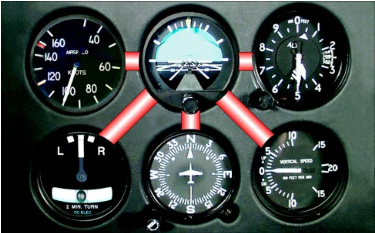
Figure 6-1. In most situations, the cross-check pattern includes the attitude indicator between the cross-check of each of the other instruments. A typical cross-check might progress as follows: attitude indicator, altimeter, attitude indicator, vertical speed indicator, attitude indicator, heading indicator, attitude indicator, and so on.
